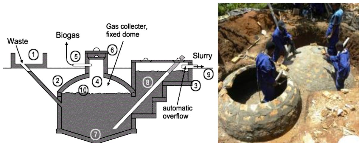
Figure 9: Fixed dome biogas plant (left)
