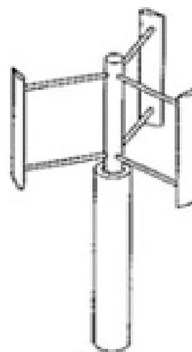
Figure 8: Darrieus Vertical Axis Wind Turbine (Source: [www.ecosources.info](http://www.ecosources.info)) (right)
