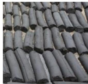
Figure 3: Briquettes made by hand from charcoal waste (left)
