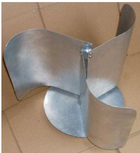
Figure 7: Savonius Vertical Axis Wind Turbine (Source: [www.reuk.co.uk](http://www.reuk.co.uk)) (middle)
